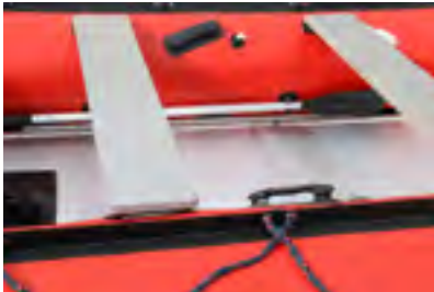
Aluminium fold away floor
