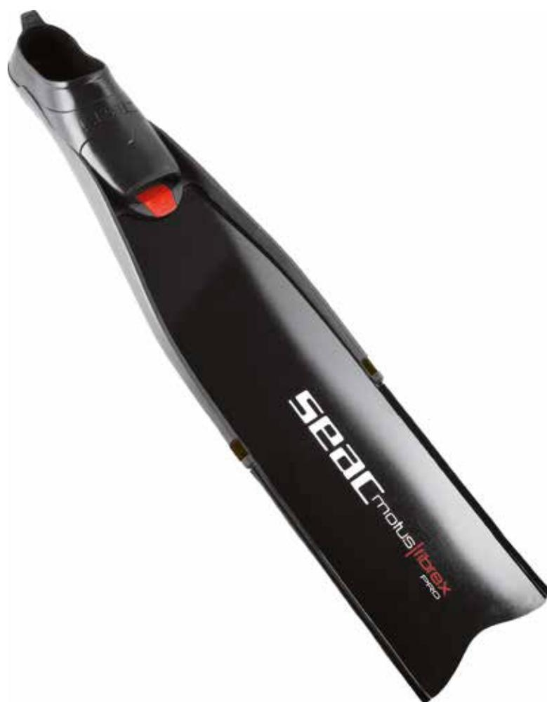
**Model:** fin with interchangeable blade and closed shoe in two materials • **Shoe material:** in double dual-density material Hard thermoplastic rubber for the sole and ribbing, soft for the shoe so as to optimize the comfort/performance ratio • **Blade material:** made with an innovative Reactive Fibreglass compound with extremely high performance characteristics.
